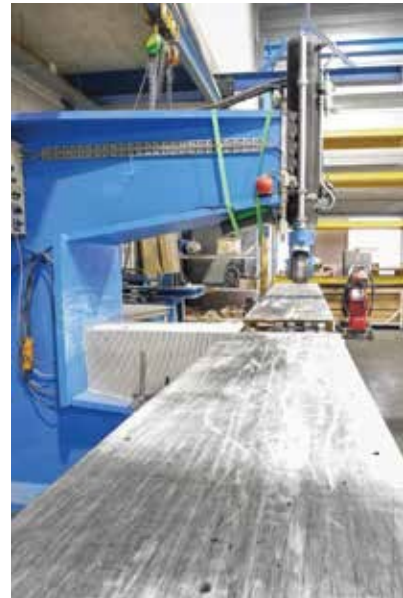
A roller is used to form the outer shell plates in a controlled manner.
