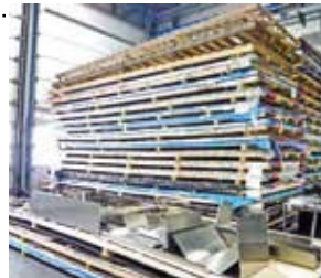
Aluminium must have the right alloys as a sheet material, but also as a profile workpiece, in order to be suitable for boatbuilding.
