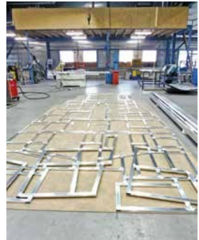
All individual parts of the floor are spread out on the ground before installation.
