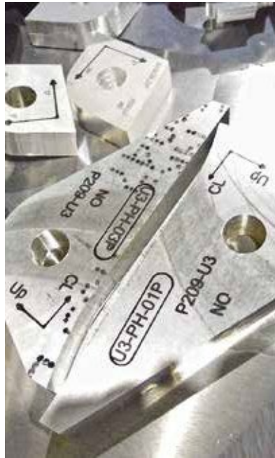
Each individual component is unambiguously labelled.
