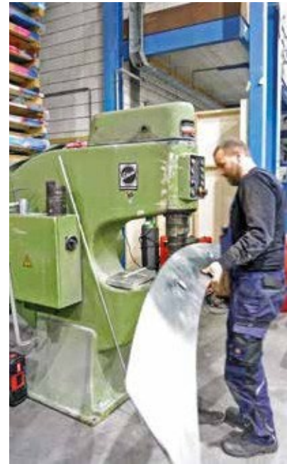
The components are shaped using a hydraulic ram.
