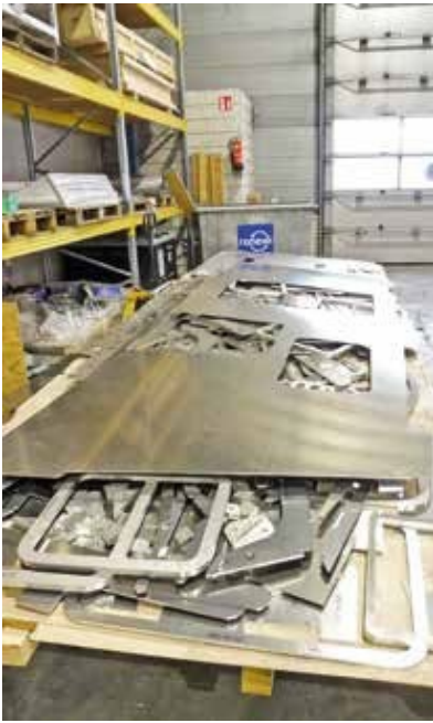
The boatyard receives ready-cut panels and components.
