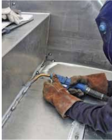
The "pilger" step procedure can be seen as the welder pauses in his work.
