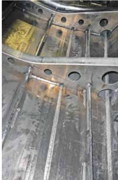
The floor timbers also have relief holes and welding holes.
