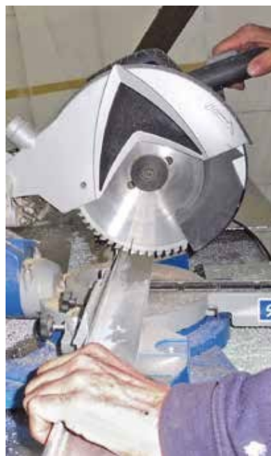
Cutting a profile to length with the cross-cut saw.
