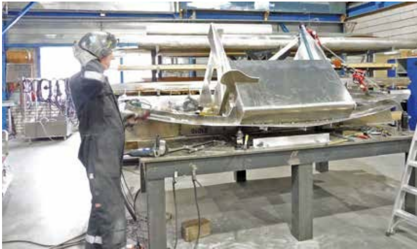
It is tried and tested practice not to build the mirror directly together with the hull, but only to assemble it as an entire component and to weld it in a precisely aligned manner.
