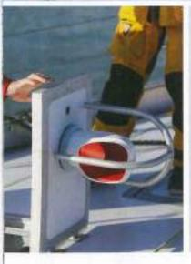
Above: handholds built into the deck saloon coaming with engine room air intakes beneath. Left: ventilation is critical in all climes. Good access to dorade box, and cowls are protected to prevent rope snagging
