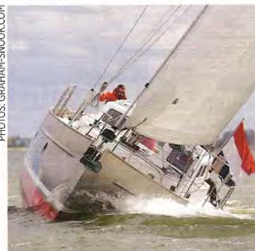
Her plumb bow maximises waterline length and interior volume
