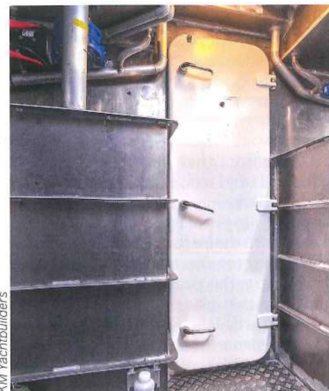
Collision bulkheads, watertight doors and plenty of stowage space aboard the new 66ft Qilak designed by Owen Clarke Design and built by KM Yachtbuilders
