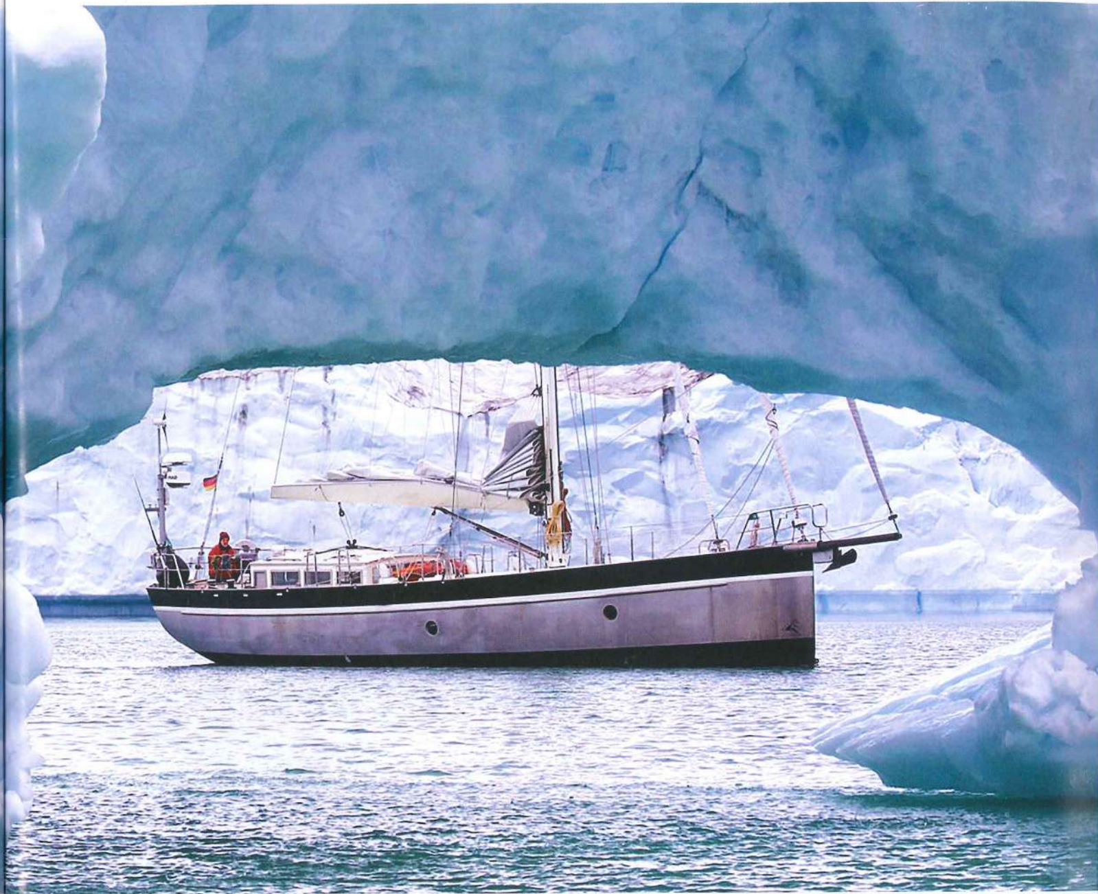
Morning Haze is an aluminium-hulled Bestevaer 55ST built specifically for high latitudes cruising
