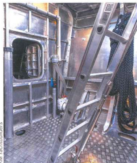
Collision bulkheads, watertight doors and plenty of stowage space aboard the new 66ft Qilak designed by Owen Clarke Design and built by KM Yachtbuilders
