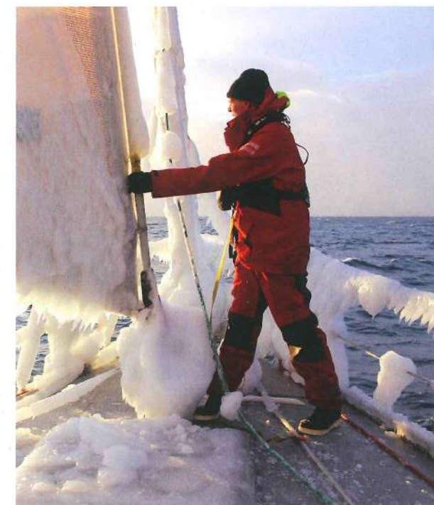
Above: this forepeak is a storage area for stores, spares, vegetables, tender and shore gear. Left: heavy ice build-ups need regular removal to maintain boat stability
