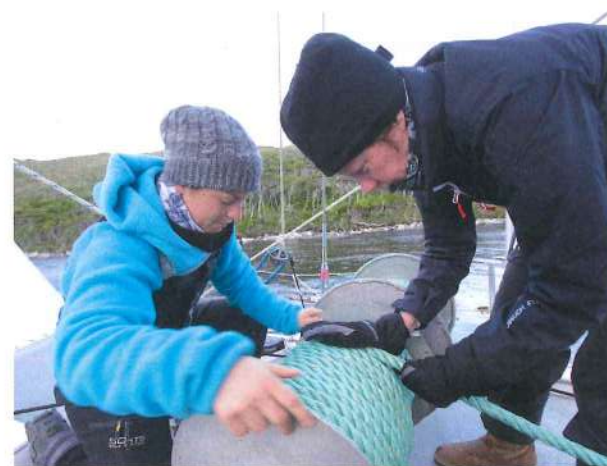
Above: if you have the space on deck, drum reels are an effective way to stow and deploy polypropylene shore lines.
